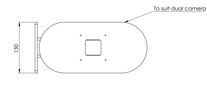
UNLESS OTHERWISE SPECIFIED: DIMENSIONS ARE IN MILLIMETERS PROPRIETARY AND CONFIDENTIAL THE INFORMATION CONTAINED IN THIS DRAWING IS THE SOLE PROPERTY OF SEE SECURITY PTY LTD. ANY REPRODUCTION IN PART OR AS A WHOLE WITHOUT THE WRITTEN PERMISSION OF SEE SECURITY PTY LTD IS PROHIBITED. FINISH: SIGNATURE DATE NAME 14/10/2016 DRAWN ADC MATERIAL: Weight 3.2kg Steel galvanised
