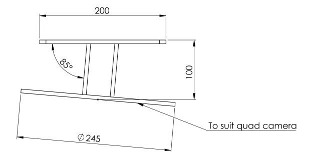
UNLESS OTHERWISE SPECIFIED: DIMENSIONS ARE IN MILLIMETERS PROPRIETARY AND CONFIDENTIAL DEBUR AND BREAK SHARP EDGES THE INFORMATION CONTAINED IN THIS DRAWING IS THE SOLE PROPERTY OF SEE SECURITY PTY LTD. ANY REPRODUCTION IN PART OR AS A WHOLE WITHOUT THE WRITTEN PERMISSION OF SEE SECURITY PTY LTD IS PROHIBITED. FINISH: SIGNATURE DATE NAME DRAWN ADC 14/10/2016 MATERIAL: Weight 3.2 kg Steel galvanised
